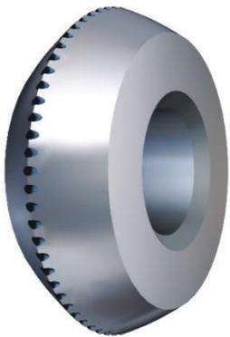
Due to its patented wheel structure with small notches, the Penett® wheel creates a very deep median crack of up to 90% of the glass thickness, which effectively simplifies or even eliminates the breaking process.
